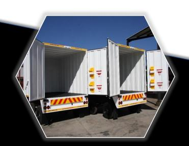
BUS TRAILER FOR USE FOR LUGGAGE TRANSPORT Rico Trailers South Africa has designed and manufactured a Bus trailer that is made for the luxury busses to use for local and cross border use. The trailer has been designed to carry the weight of the luggage so that the bus does not take the strain of the weight by carrying it and only pulls the weight such as a horse and carriage does. This allows for maximum efficiency for both the bus and trailer.
